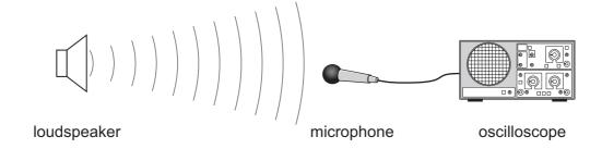
Yuri connects a microphone to an oscilloscope.
